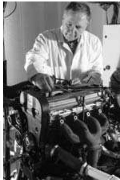
An engine is being readied for testing on a dynamometer
