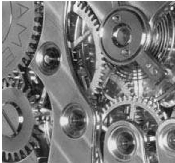
Gear trains inside a mechanical watch
